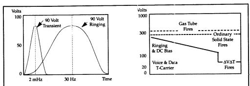
$\Delta V/\Delta T$  technology reads the rate of rise over time to determine if the low level voltage should be filtered out. A 90 volt ringing current has a very slow rise when compared to that of a transient and is easily differentiated. Fast edged transients as low as 50 volts are filtered out using this technique.
